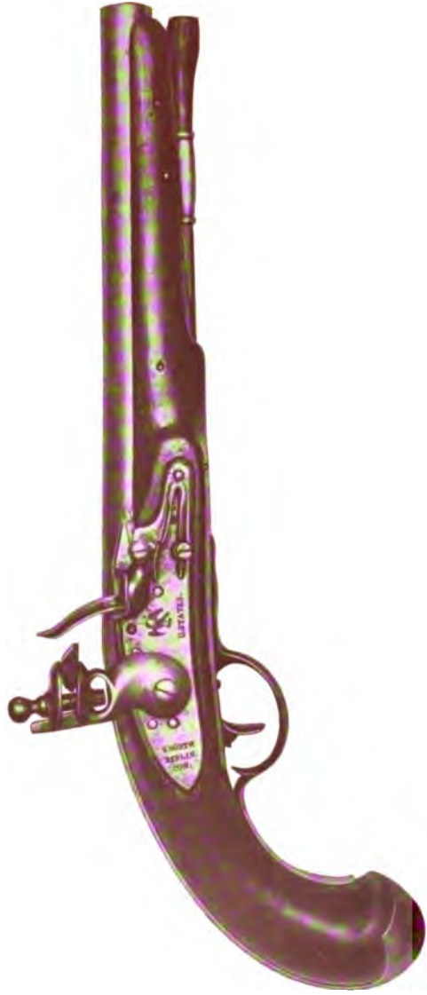
Navy pistol; model of 1808. Length 16½ inches. Length of barrel 10½ inches. Caliber about 64. Iron belt hook for use of sailors in boarding. Brass mountings.
